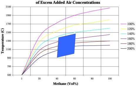
Flame Temperature (C) for CH<sub>4</sub>/CO<sub>2</sub> Gas Mixture for a Range of Excess Added Air Concentrations
