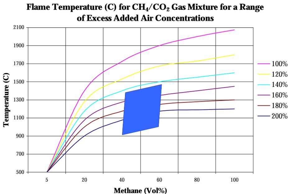
flares usually operate at the right hand side of the envelope at CH<sub>4</sub> >50% with the excess air to biogas ratio of the order of 10-15 volumes of air : biogas. Under these conditions the air is employed to both oxidise the biogas and cool the flame – it also propagates more turbulence and mixing. Mixing within the burn is crucial to ensure that all the biogas is burned uniformly and under ideal conditions.
